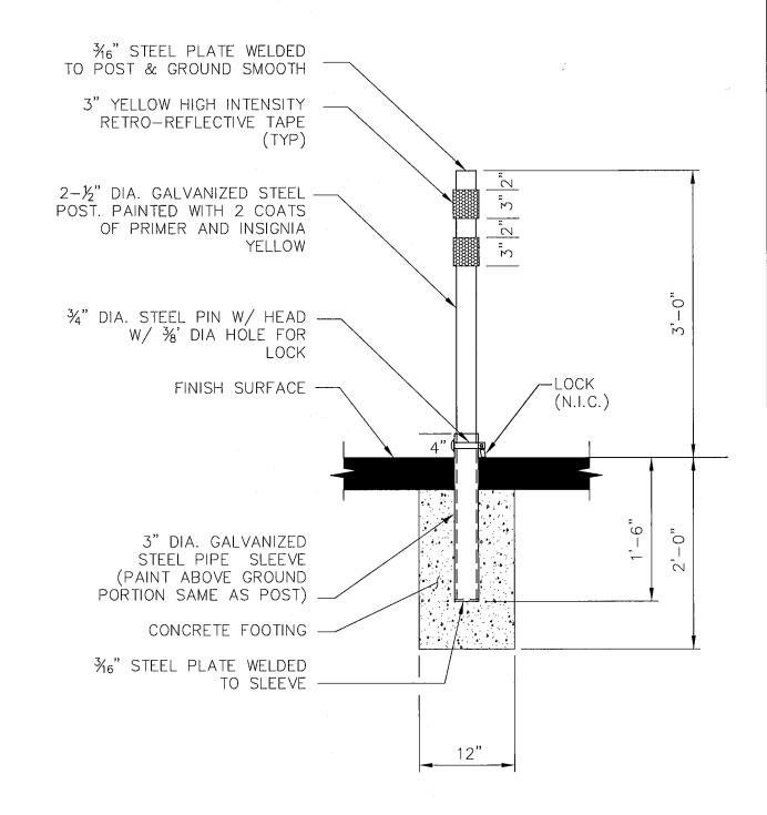
NOTE: DRILL A  $^{13}\!\!/_{6}$ " DIA HOLE THRU BOTH THE POST AND SLEEVE FOR PIN PLACEMENT
